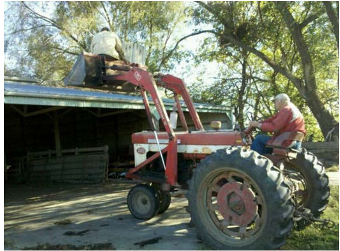
Figure 4. Front end loader being used as a lift. This is a very dangerous situation, and loaders should never be used in this manner.
