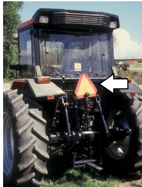
Figure 3. Slow moving vehicle (SMV) emblem. The SMV emblem should be mounted at the rear of any vehicle or towed equipment traveling less than 25 mph.
